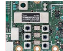
1.2kHz Optimum Roofing Filter 3, 6, 15kHz High-Spec 1st IF filters
