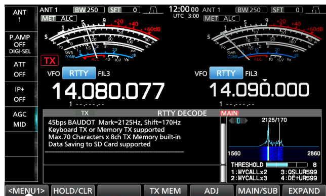
RTTY DECODE screen <MENU1>
